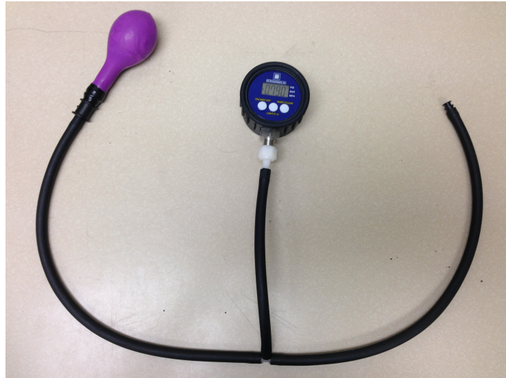
Figure 3.2: Device created to simulated a loaded fluid filled deformable pressure vessel such as the eye
